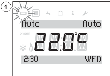
Fig. 17 Low battery indication
