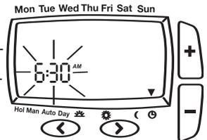
Once you have selected your required display, to adjust press + or - and > to accept change. To select option 06 press > until option 06 display is shown
