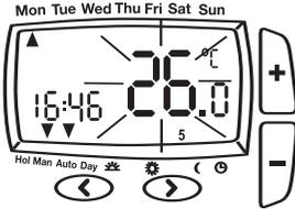
2. After 5 seconds will start controlling at selected set point but displays actual room temperature. Two chevrons indicates override mode.
