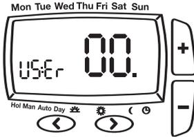
**NOTE: To exit User Options press < and > simultaneously for 3 seconds.**
