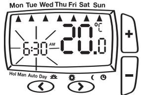
2. Once the time has been set press > to confirm and use + or - button to adjust required temperature (temperature \*shown flashing)
