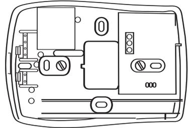
2. Fix the back plate directly onto the wall using suitable wall plugs and screws.
