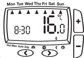
4. To exit press < or > until you return to auto mode with the bottom arrow pointing to auto (as shown).
