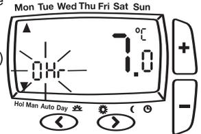
2. Press + or - buttons to adjust the count down time as required. Press > once to confirm, the display will show temperature flashing.
