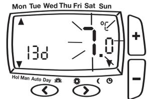
3. Press + or - buttons to adjust temperature and press > to start holiday count down time. Alternatively after 10 seconds the temperature will stop flashing and holiday count down time will start. Display shows count down time and ambient room temperature.
