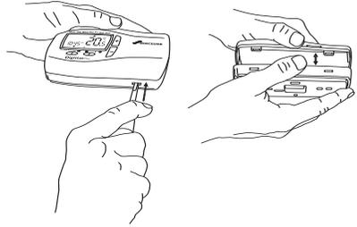
1. Remove the front cover using a flat screwdriver and separate from back plate.
