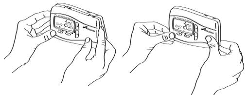
3. Replace the front cover by locating in position and pushing fully onto the back cover.
