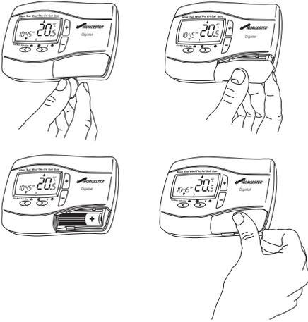
4. Remove the battery cover using a coin (Fig 4).
