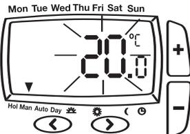
2. Press + or - buttons to adjust the temperature as required. The temperature will stop flashing after 5 seconds and start controlling at this temperature.
