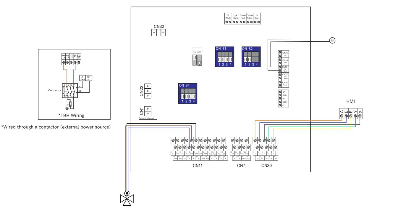
If a third party diverter valve is used wiring and orientation may differ. Seek advice for compatible products
